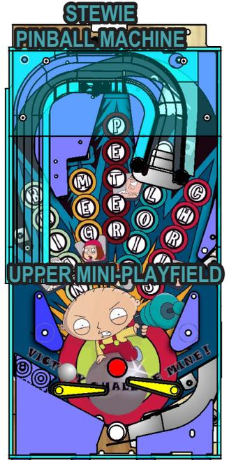
The 'baby' (Stewie) version of a pinball game inside the large one. This is referred to as the upper mini-playfield. The ball on this playfield is half the size of the normal steel ball. Spell out B-R-I-A-N (left orbit), M-E-G (stand-up target), P-E-T-E-R (stand-up target), L-O-I-S (ramp shot and C-H-R-I-S (right orbit) by completing each shot.
