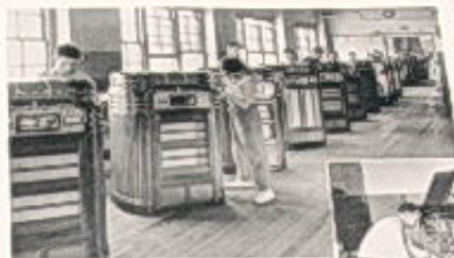
Final Inspection Under the sharp eyes of a trained inspector, a Symphonola is put through a final examination. Lighting, cabinet construction, tuning performance and amplifying system must prove flawless before it is pronounced "O. K."
